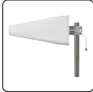
698-2700 MHz Low Pim Log Periodic Antenna
