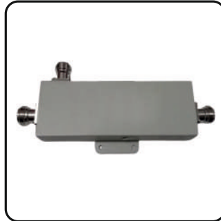
550 - 6000 MHz Low Pim 5 dB RF Directional Coupler
